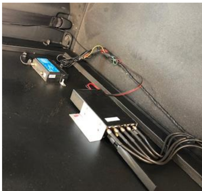
Figure 25. In-car LTE router installation
