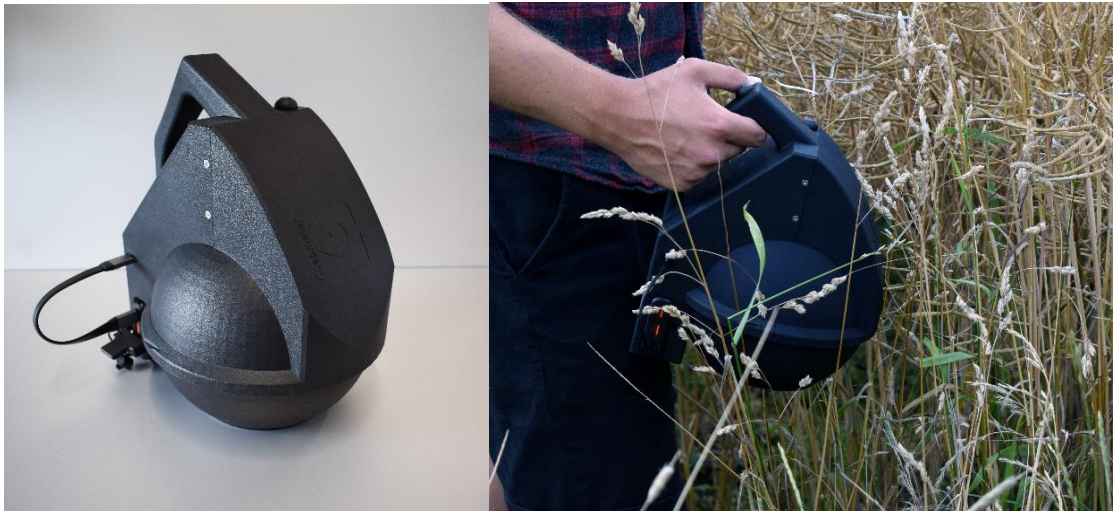
Figure 1. VideometerLite, portable handheld spectral imaging device.
