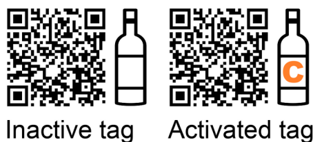
Figure 4. Smart tag design that consists of a QR code and letter code printed in photosensitive invisible ink.
