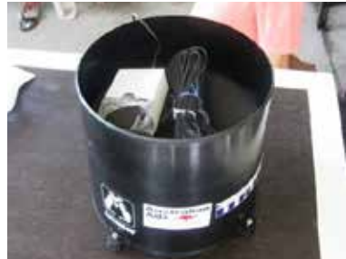
A Digital Rain Gauge used to measure rainfall. With technical assistance, communities can correlate amount with rainfall and flooding which then will be the basis for the early warning information.
