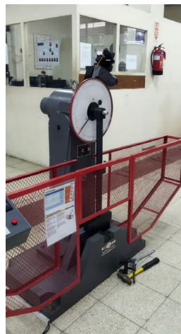
Fig. 2. The impact toughness test machine
