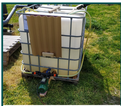
Figure 2: Bioextractor and aeration device to produce compost tea directly in the farm
