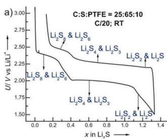
Unlike the intercalation in Li-ion cells, the Li-S cells have progressive chemical reactions that start from the elemental Sulphur (cathode) and then transform into polysulphides of different combinations with Lithium. These polysulphides travel between the electrodes, hence creating the shuttling effect [4]. The highly nonlinear characteristic curve with two distinct plateaus creates a great challenge for modeling.
