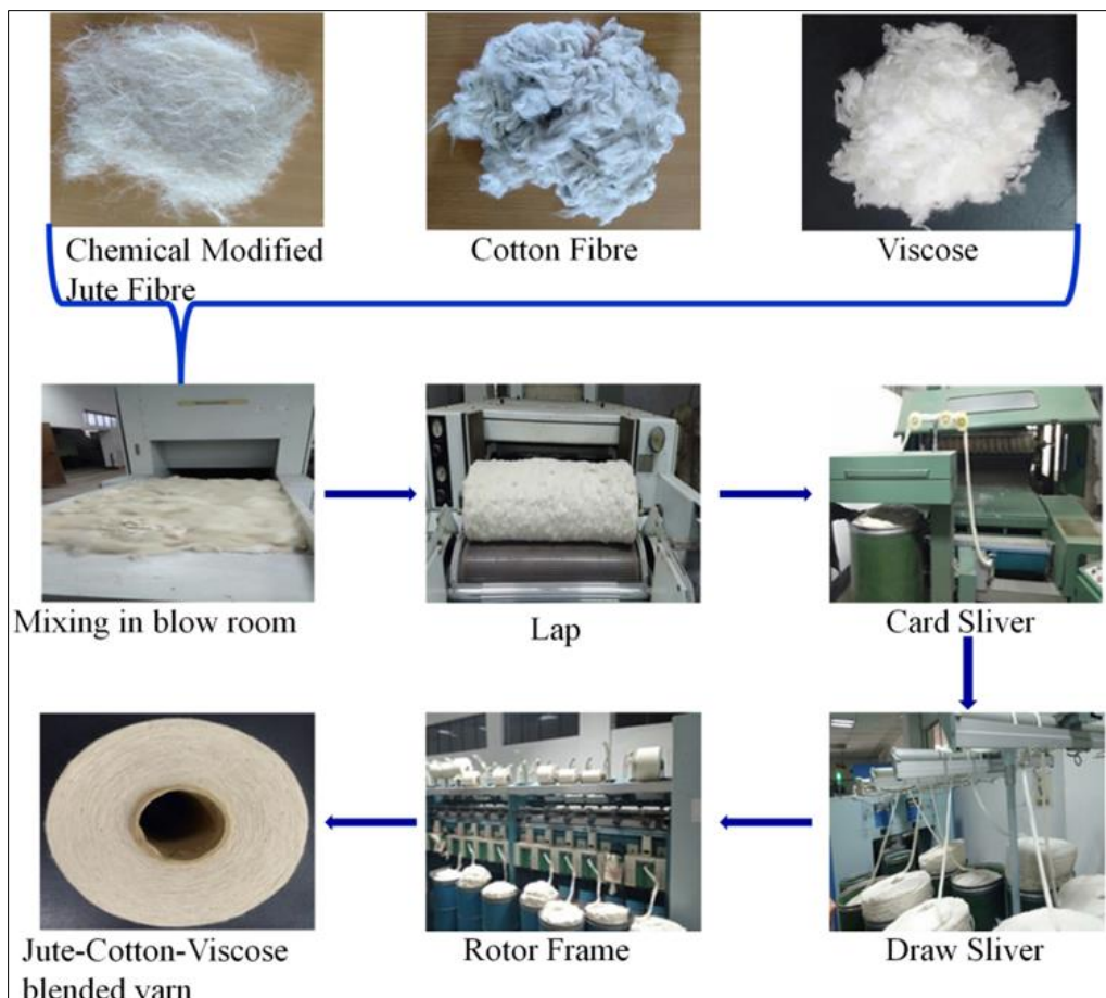
Figure 2 Flow chart diagram of blending process
