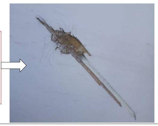
This damage is at 80% span on the suction side shell.
