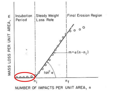
coating mass loss < 10% laminate mass loss = 0%
