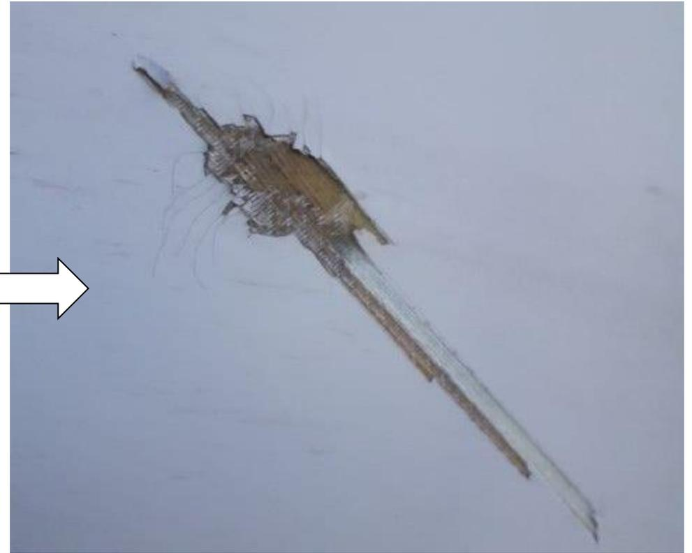
This damage is at 80% span on the suction side shell.
