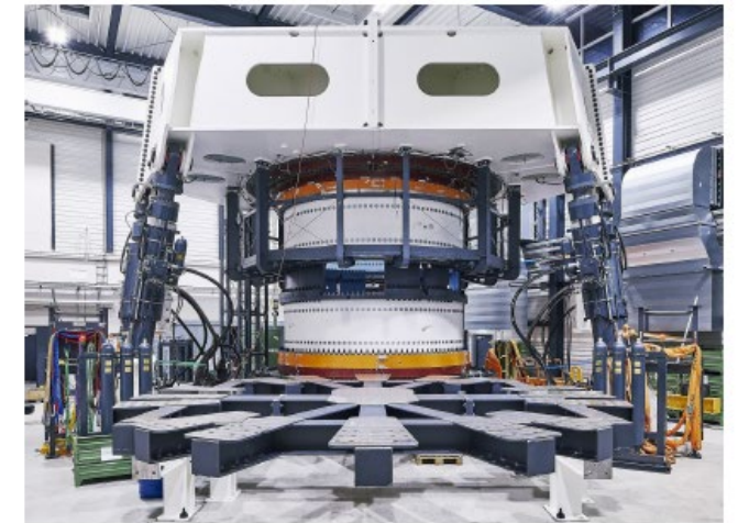
(d) "BEAT6.1", for 5 m bearings (in orange) ©Fraunhofer IWES/Marcus Heine
