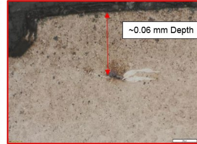
White structure found near the fracture and raceway surface, Magnification: 500x
