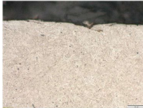
OR raceway surface cracks and peeling
