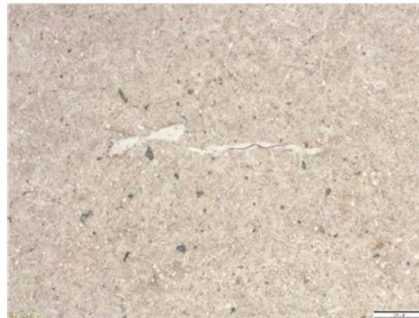
White structure below the raceway surface, Magnification: 500x
