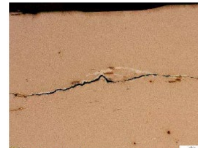
GS roller surface, magnification: 50x
