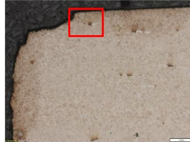
Circumferential cut of the fracture surface, Magnification: 100x
