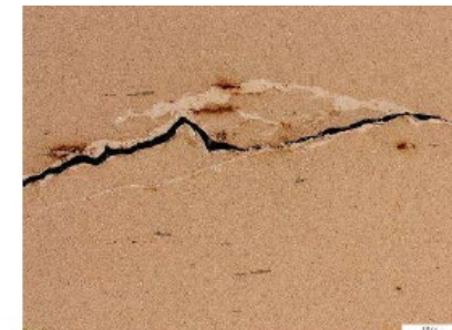
White structure and cracking, magnification: 100x
