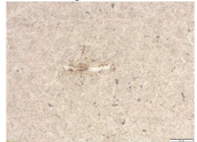
White structure below the raceway surface, Magnification: 500x
