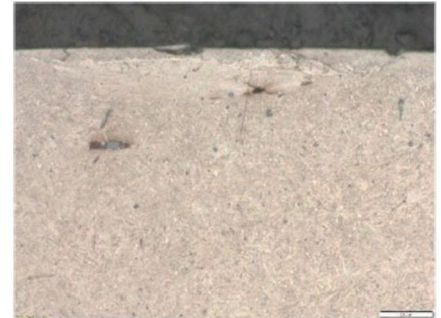
White structure on the raceway surface, Magnification: 500x
