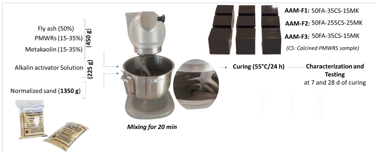
Fig.1. Alkali activated mortars AAMs preparation protocol.
