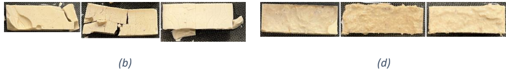
Figure 13. Images of plain, (a) and (b), and fibre reinforced, (c) and (d), alkaline activated geopolymer after freeze-thaw cycles.
