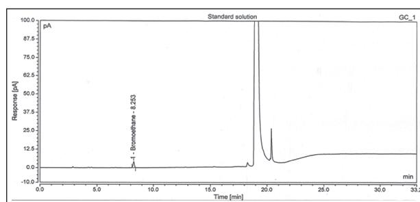
Figure 4. Typical chromatogram of standard.
