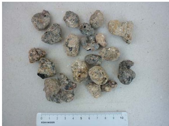
Fig.2: Clay lumps from US779 (sample 85)
