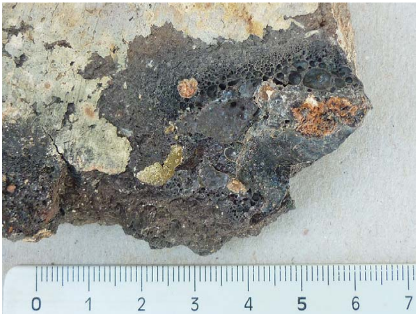
Fig.13b: Particular of vitrification on the internal surface (sample 115 b)
