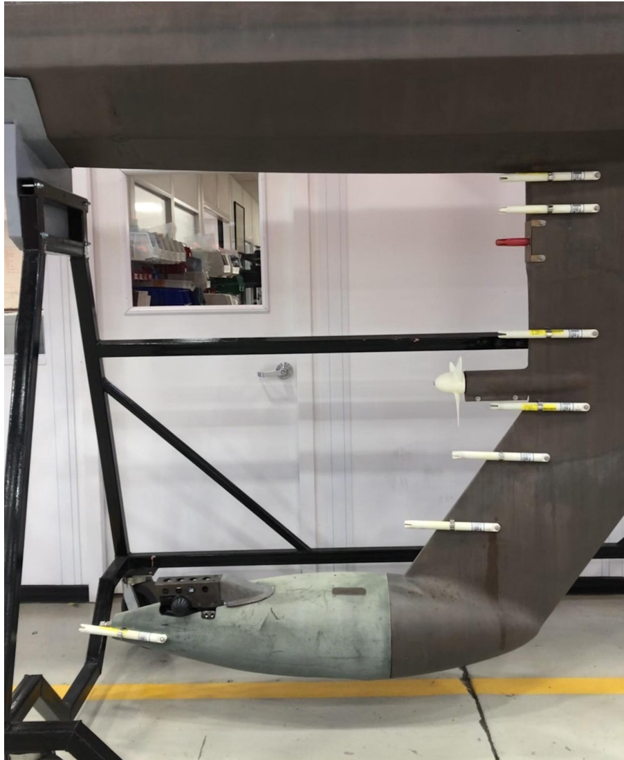
Figure 3. Seven Seabird SBE56 temperature loggers were mounted on the keel at depths specified in Table 5. Image credit: Saildrone, Inc.
