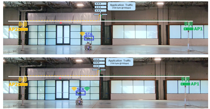
Fig. 8. Roaming experiment scenario with Mobile Robot in a warehouse environment
