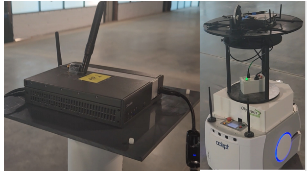
Fig. 9. AP implemented as a NUC operating as soft-AP and Mobile Robot with mounted NUC
