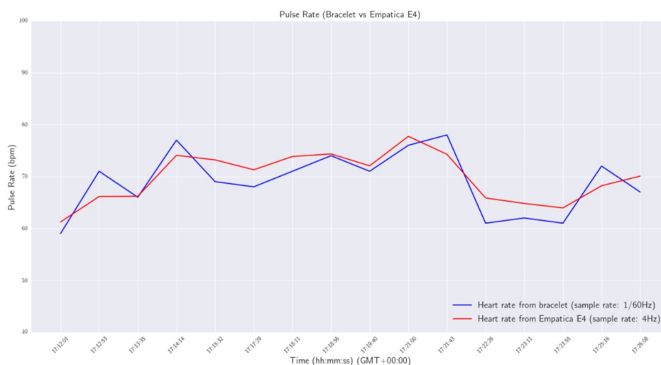
Figure 9. Pulse Rate - Smart wristband vs Empatica E4.
