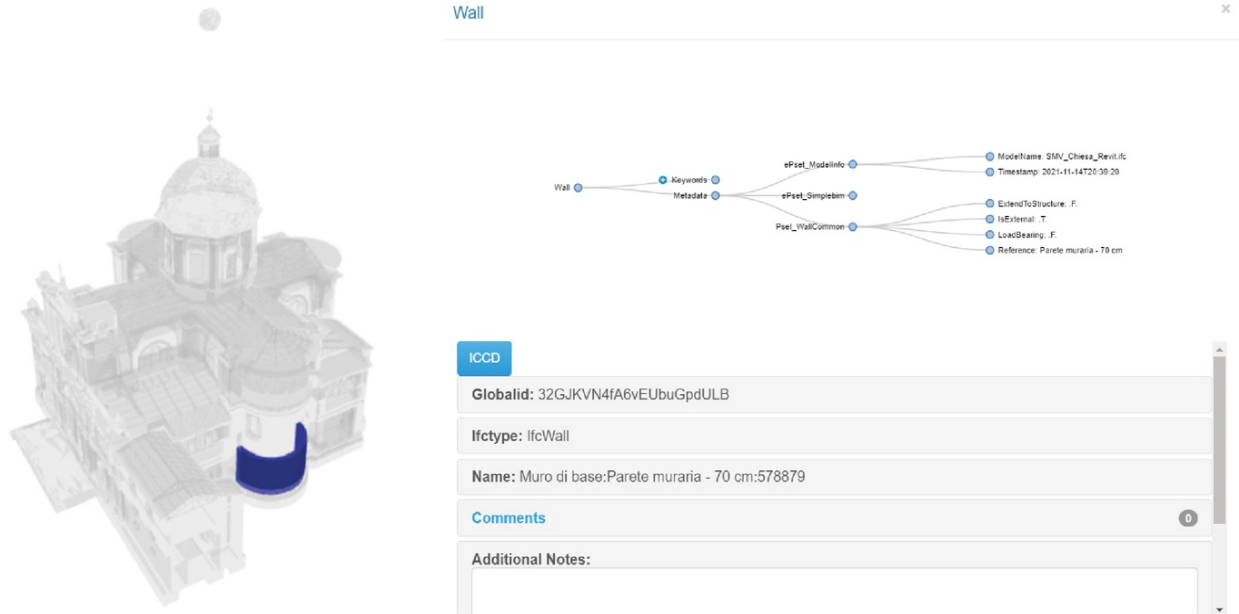
Figure 4: Every element of the building can be used to perform a live SPARQL query that returns all the details for that element, according to the HBIM ontology. Each value can be updated via web, thanks to the SPARQL 1.1 Update functionalities.
