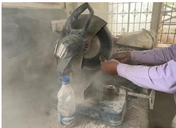
Figure 6. Cutting of the sample for WCA measurement
