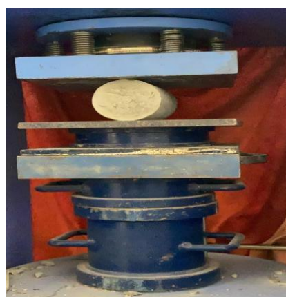
Figure 5. Testing of cylinder by CTM for split tensile strength
