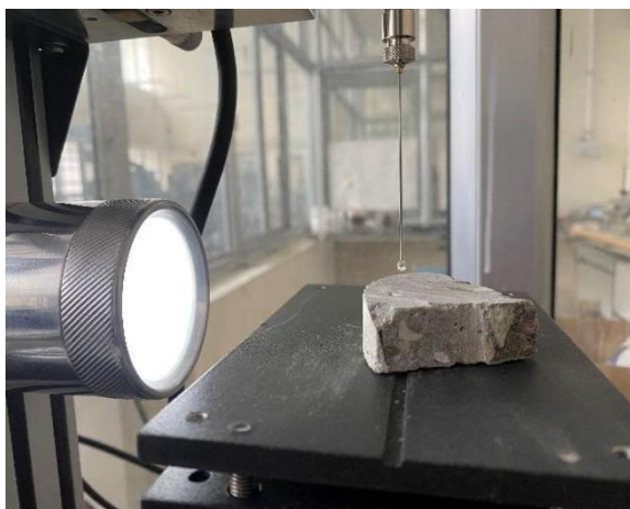
Figure 8. Dispensing the water droplet from the Syringe onto the concrete specimen
