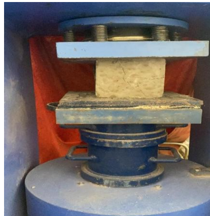
Figure 4. Testing of cube in CTM showing the failure of the sample
