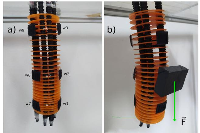
Fig. 1. (a) A single module of the I-support arm in relaxed condition. The locations where the external load will be placed are shown and labeled  $w_1, w_2, \dots, w_9$ . (b) The arm with an external load placed on location 2.
