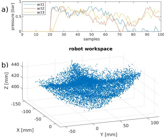
Fig. 2. (a) The first 100 samples of quasi random actuation inputs provided to the robot for motor babbling. (b) The robot workspace recorded with an NDI Aurora electromagnetic tracking system during a motor babbling session.
