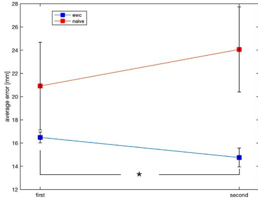
Fig. 9. The average cartesian error on the first round of weights compared to the average error for the second round of weights, for the EWC and naive methods.
