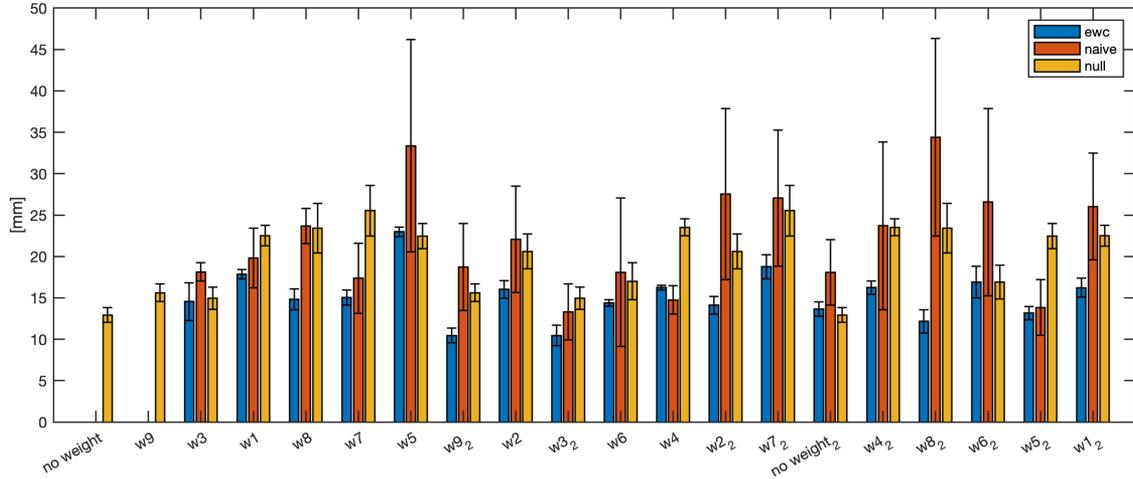
Fig. 5. The mean task space error computed for each trial shown for the EWC, SGD (naive) and null methods after training only on previous loading conditions, and before retraining on the current condition. On the x-axis the conditions  $w_1, w_2, \dots, w_9$  are indicated, while the subscript  $w_{1_2}, w_{2_2}, \dots, w_{9_2}$  indicates that the condition is encountered the second time.
