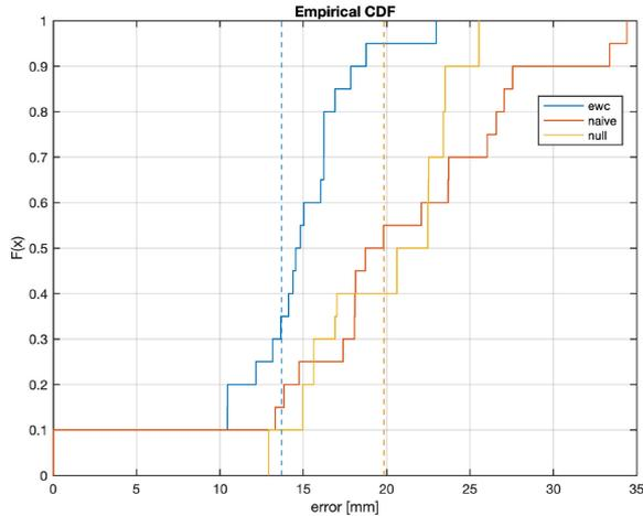
Fig. 6. The cumulative density function plots of the Cartesian kinematic errors from change in loading before network retraining for the new load. The dashed lines represent the mean of each distribution.
