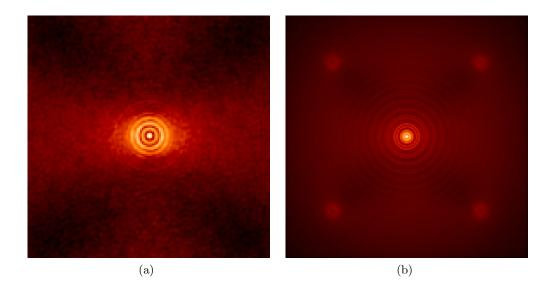
Figure 3. Simulated images of AU Mic. a) is with the classical Lyot coronagraph, while b) is the off-axis PSF used for contrast normalization.
