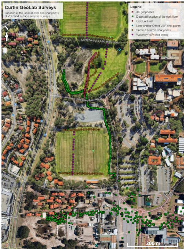
Figure 1. The Curtin In-Situ GeoLab VSP and surface dark fibre surveys acquisition map. Red dot – location of the GeoLab well. Blue dots – location of the near and far VSP offset shot points. Purple dots – locations of the walkaway VSP shot points. Pink dots – location of 3C geophones. Orange dots – locations of the surface seismic (dark fibre) survey. Green dots are determined locations of the dark fibre.
