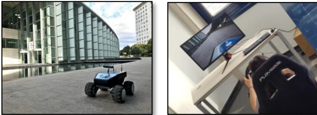
Figure 6: Illustration of remote driving concept of an AGV vehicle ( https://fivecomm.eu/ )
