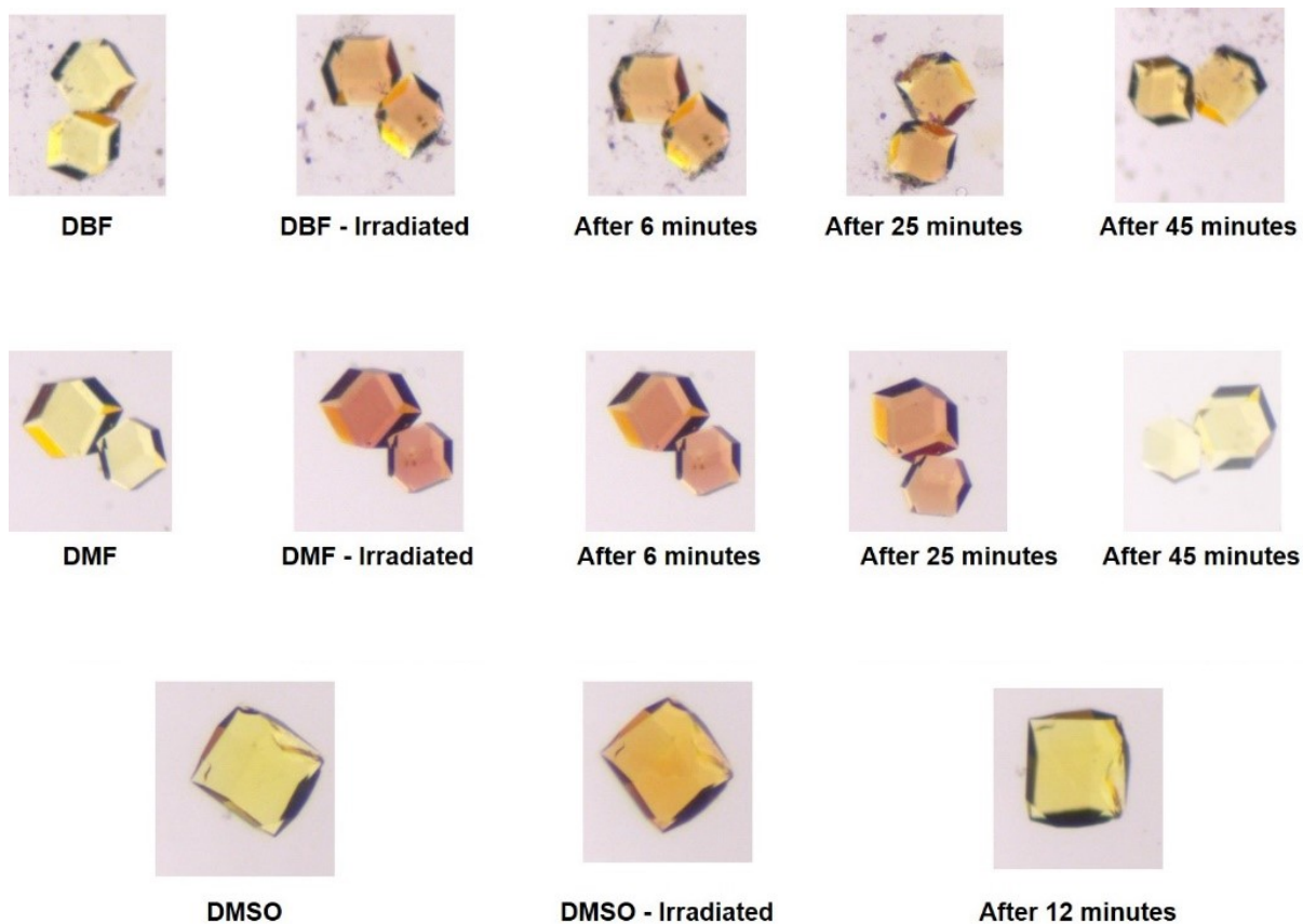
Figure S9: Crystals of MUF-77-bdc-paq suspended in N,N -dibutylformamide (DBF), N,N -dimethylformamide (DMF), and dimethylsulfoxide (DMSO) at different time intervals after irradiation with a 405 nm laser pointer for 10 seconds.
