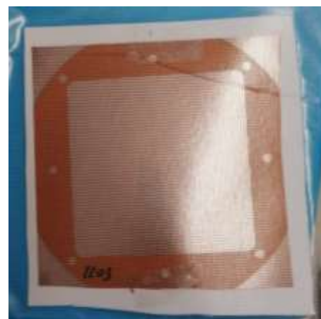
Fig. 8 Left: Vacuum equipment to prevent the top Cu layer from oxidation: vacuum sealer for domestic use and a first 6x6 cm 2 DLC-Cu deposition sealed in a vacuum bag. Right: first 10×10 cm 2 DLC-Cu deposition sealed in vacuum.
