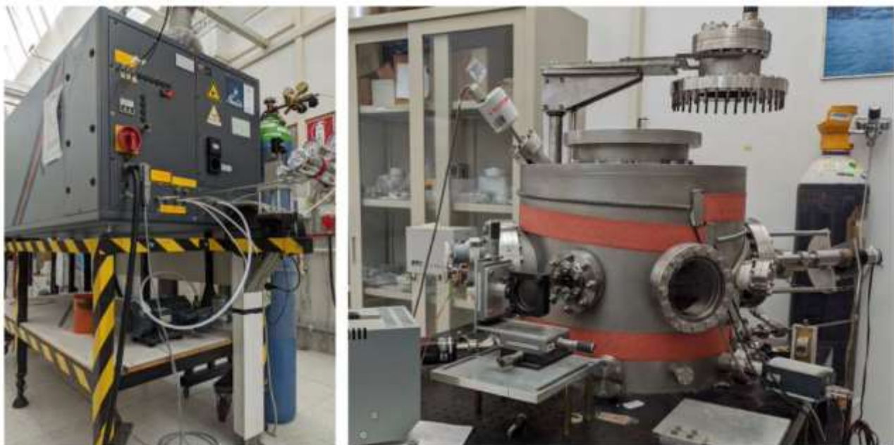
Fig. 10 PLD lab at INFN Lecce. Left: Eximer laser. Right: Vacuum vessel with (not visible) target and substrate holder.
