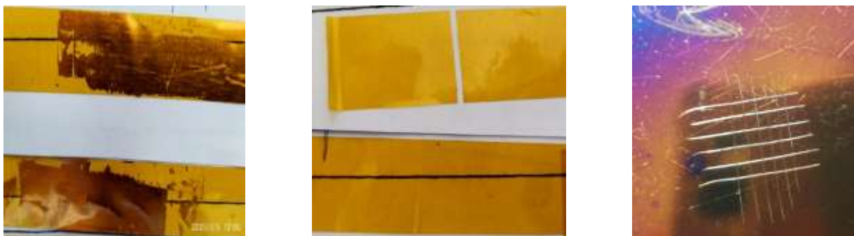
Fig. 6 Results of the scotch tape test on top of the final copper layer (50 nm). When copper is removed by the tape this indicates an insufficient adhesion, when instead no copper can be noticed on the yellow Kapton tape after the test the adhesion is good. Left: insufficient adhesion of Cu in a sample with 10 nm Aluminium interlayer (top) and a 10 nm Titanium interlayer (bottom). Middle: good adhesion of Cu obtained through cleaning of the DLC layer before the deposition of a 10 nm Titanium interlayer (top) or 10 nm Chromium interlayer (bottom). Right: results of a scratch test: no Cu was removed by the scotch tape test after vertical and horizontal cuts on the Cu top layer [15].
