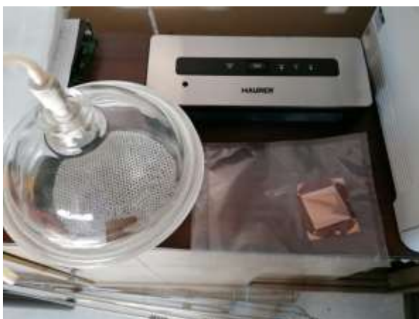
Fig. 8 Left: Vacuum equipment to prevent the top Cu layer from oxidation: vacuum sealer for domestic use and a first 6x6 cm 2 DLC-Cu deposition sealed in a vacuum bag. Right: first 10×10 cm 2 DLC-Cu deposition sealed in vacuum.
