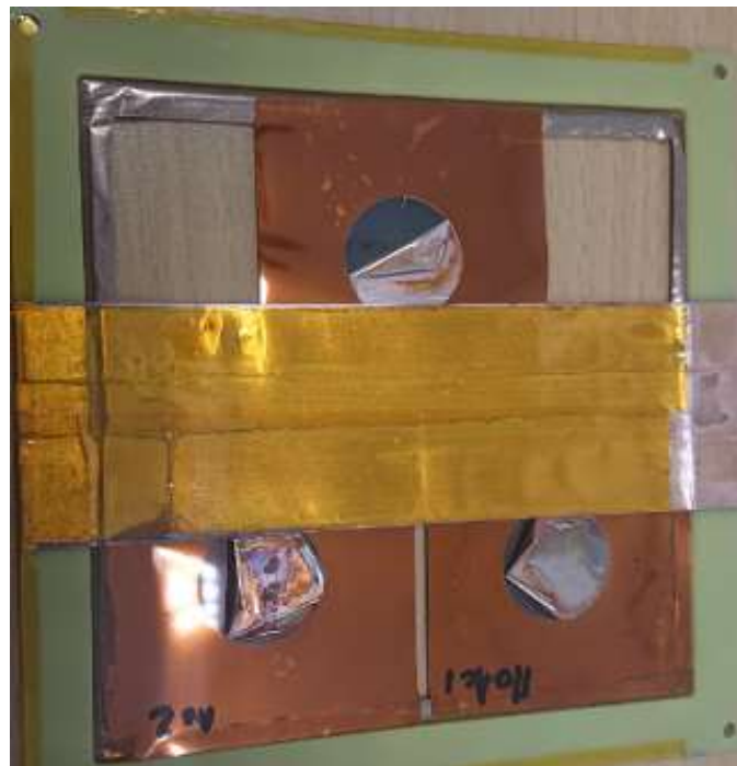
Fig. 11 The result of the electroplating of a 7 \mu m Cu layer on top of three 5x5 cm 2 PLD made Cu-Cr-DLC-Polyimide foils. One can clearly observe the delamination of the electroplated Cu layer after drying of the sample.
