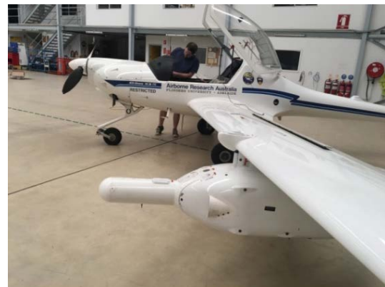
Figure 6. The wing pod mounted on the test aircraft. A GNSS antenna is mounted above the pod on the leading edge of the wing.
