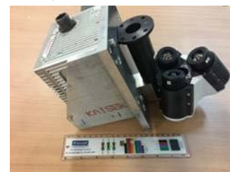
Figure 3. The NASA NDL 1'' optics and IMU bolted to a rigid aluminium frame, allowing frame transformations accurate to approximately 0.01°.
