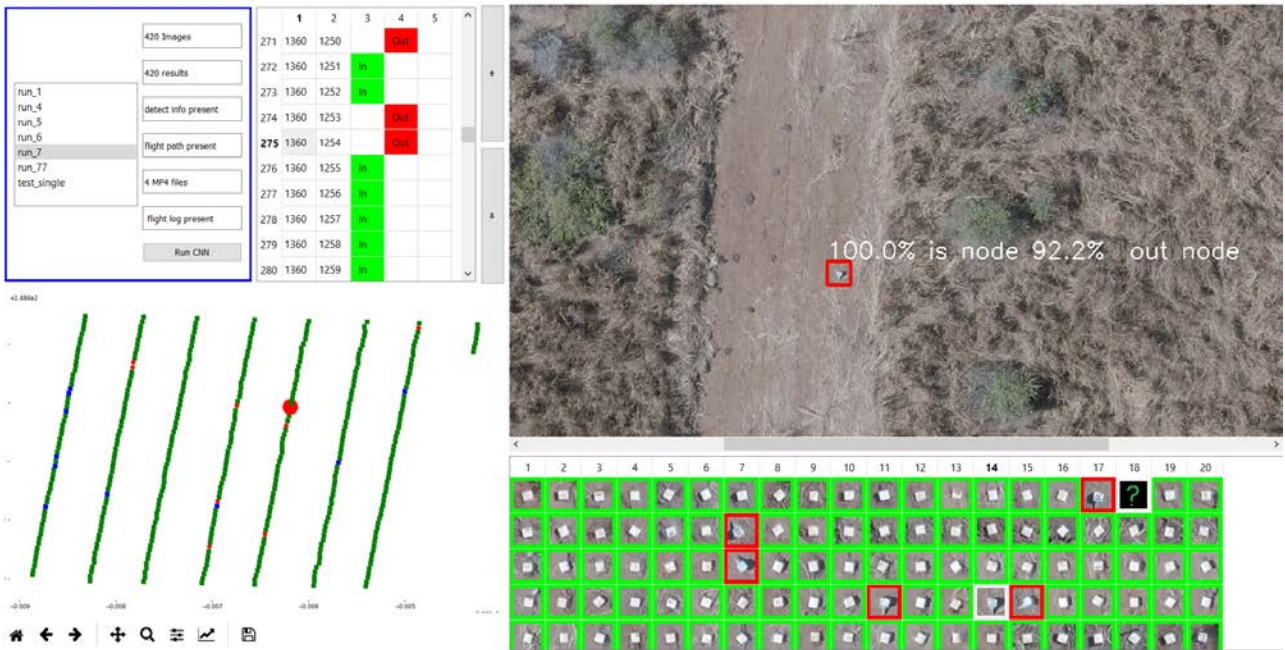
Figure 4. Display software used to view the results of the CNN analysis. (top left) table of image status. (bottom left) colour coded map of flight. (top right) selected analysis location. (bottom right) surrounding node images.
