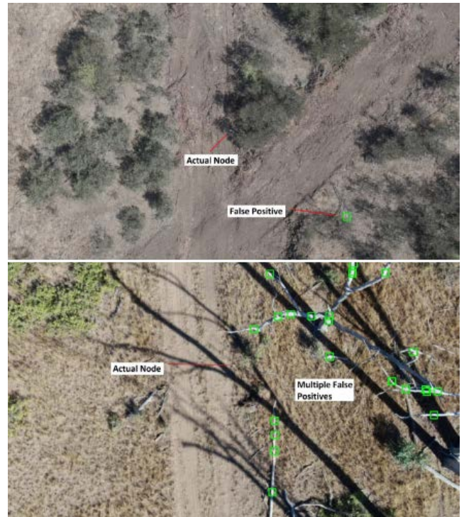
Figure 2. Examples of false node identification by OpenCV simple blob detection.
