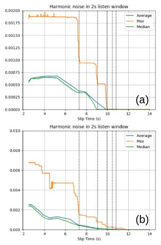
Figure 2. Comparison of the cross-harmonic noise for a theoretical sweep (a) and the ground force (derived during testing) (b). Dotted lines indicate the harmonic limits expected from theory (Pieuchot, 1984).
