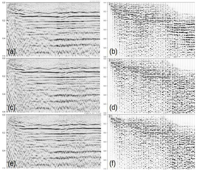
Figure 4. Comparison of the impacts of harmonic noise from slip-sweeps in good (left) and poor quality data (right). (a) & (b) traditional acquisition. (c) & (d) slip-sweep acquisition. (e) & (f) slip-sweep including CDP domain, TF median-filter burst-noise rejection.
