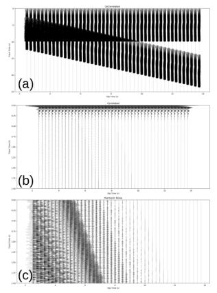
Figure 1. Presurvey estimate of slip-sweep correlation noise. Sweep parameters are linear 10-180Hz, 10s, 2s listen. (a) uncorrelated sweeps with slips ranging from 2.5s to 14s. (b) correlated traces. (c) difference between slip sweep and independent acquisition (harmonic noise).
