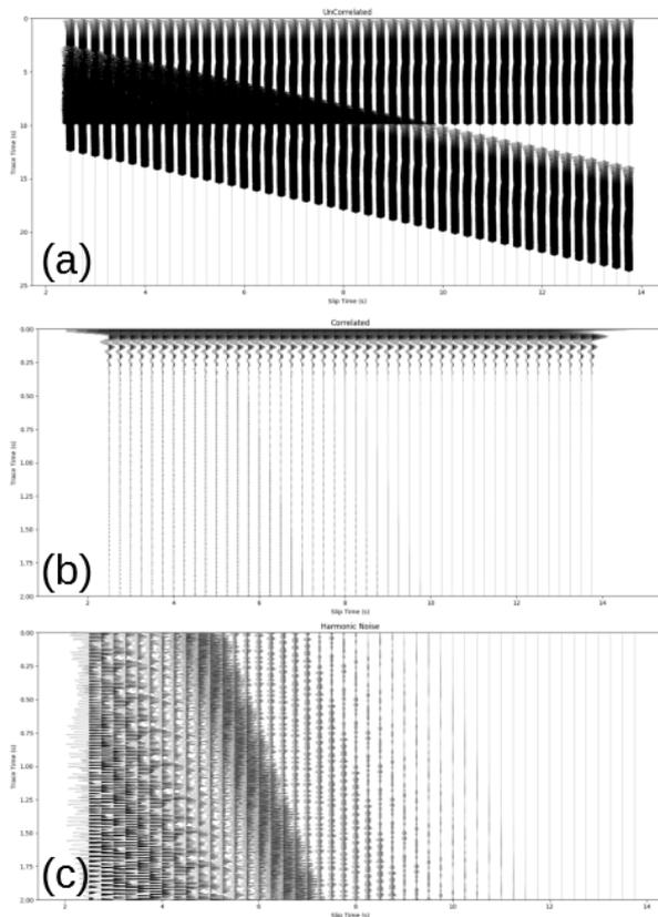
**Figure 1. Presurvey estimate of slip-sweep correlation noise. Sweep parameters are linear 10-180Hz, 10s, 2s listen. (a) uncorrelated sweeps with slips ranging from 2.5s to 14s. (b) correlated traces. (c) difference between slip sweep and independent acquisition (harmonic noise).**
