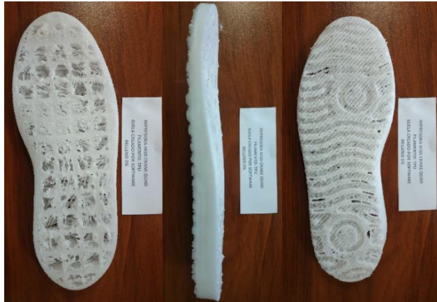
Fig. 7. Digitized sole by software design and printed with M3D Crane Quad equipment in TPU Flexible Filament with 5% infill.
