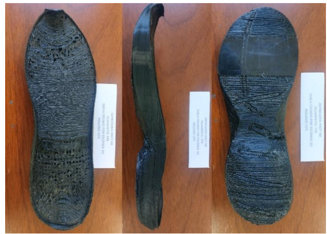
Fig. 15. Digitized sole by 3D Scanning and printed with ANET A8 equipment in TPE Flexible Filament with 12% infill.
