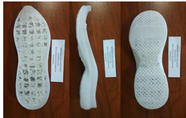
Fig. 14. Digitized sole by 3D Scanning and printed with M3D Crane Quad equipment in TPU Flexible Filament with 5% infill.
