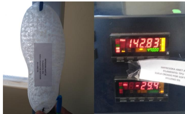
Fig. 16. Tensile and elongation test applied to the sole created by software design.
