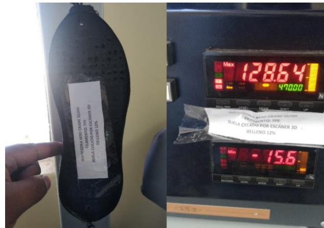
Fig. 17. Tensile and elongation test applied to the sole created by 3D Scanning.
