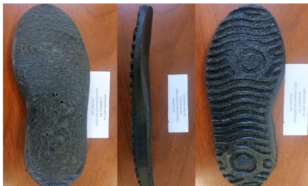
Fig. 8. Digitized sole by software design and printed with ANET A8 equipment in TPE Flexible Filament with 12% infill.
