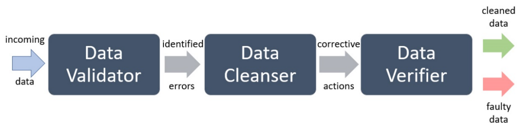
Figure 4: Data Cleaner internal workflow.
