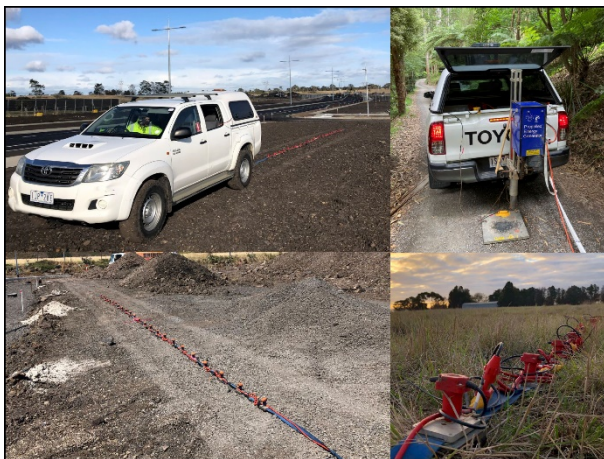
Figure 3. Site photographs of the MASW setup.
