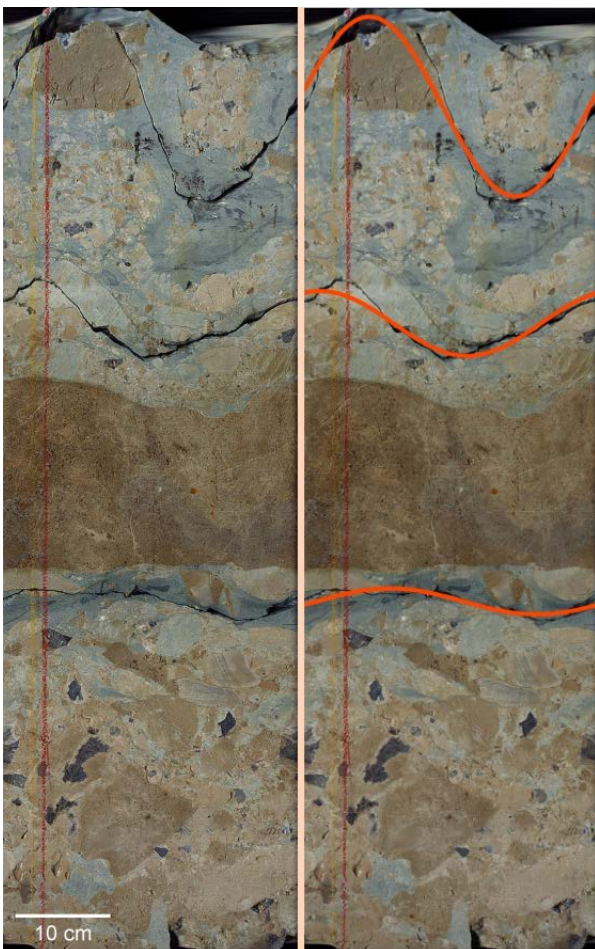
Figure 2. Fracture detection by the model, input image is shown on the left and detected fractures are shown in red on the right.
