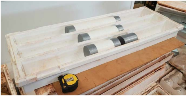
Figure 2. A sample reference tray developed for testing the accuracy of the method.
