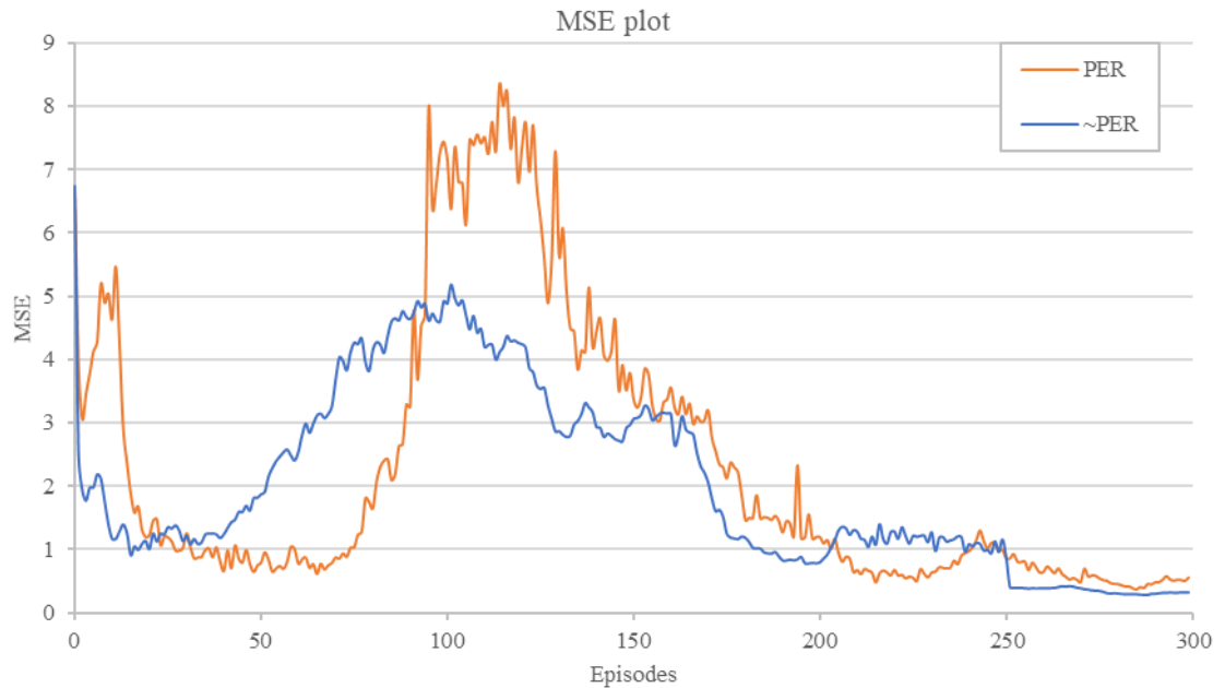
Figure 44 – the MSE of prioritized sampling compared to random sampling in the experience replay buffer.
