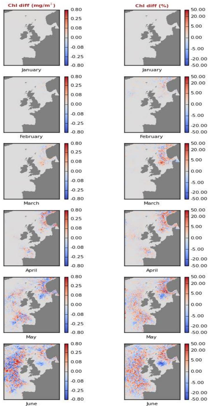
Figure 4.3.7 Impact of the glider chlorophyll assimilation in the multi-platform DA on the NWES during the Jan-June 2018 simulation period. The left-hand panels show the impact in absolute values, defined as an average monthly difference in surface chlorophyll between the multi-platform DA run and the run assimilating only satellite data. The right-hand panels show the same as left hand panels, only relative to the surface chlorophyll value (in %). The different rows show different months.
