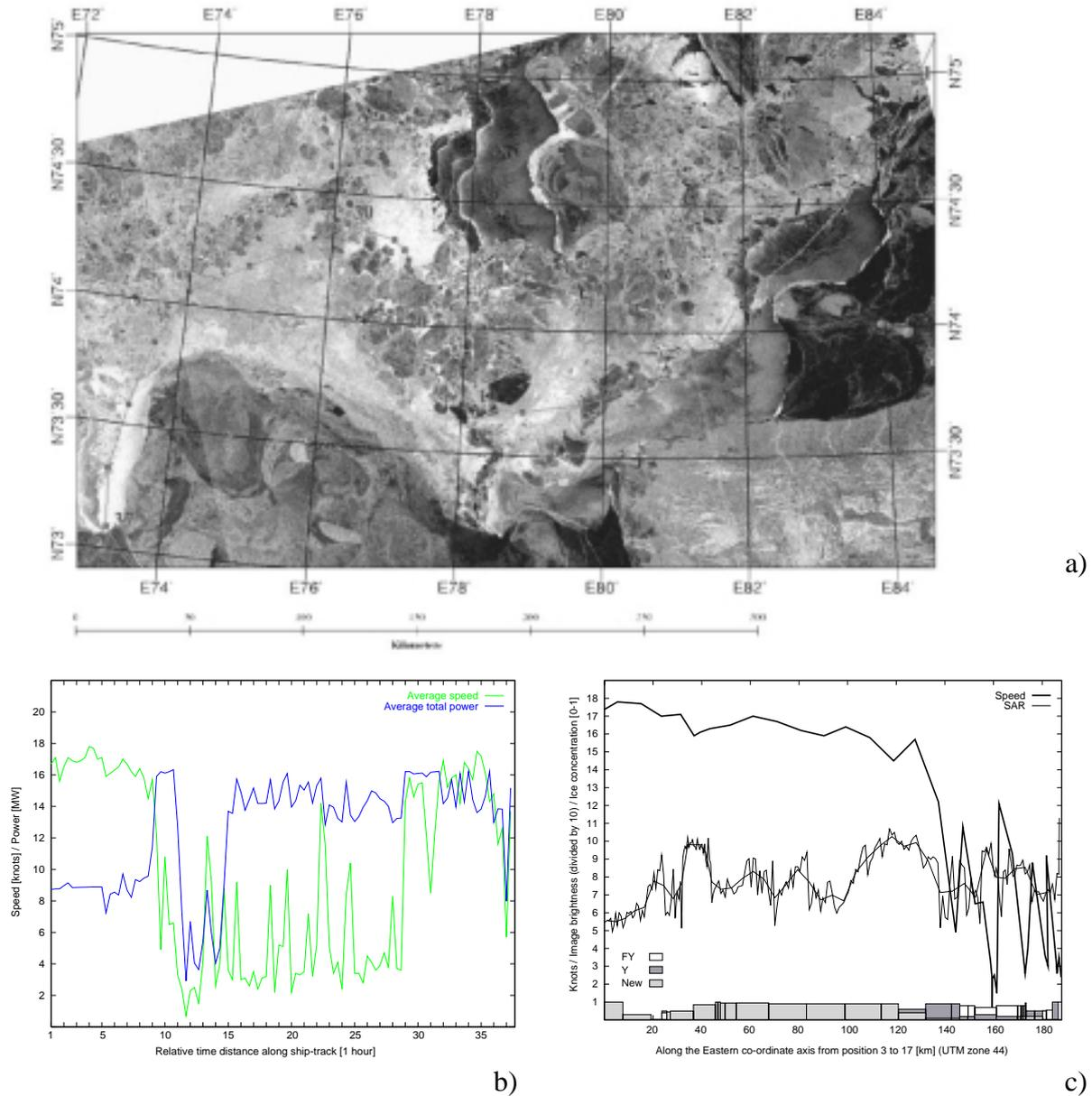
Figure 35. a) Sub-image of RADARSAT ScanSAR of April 30. Superimposed in green is the ship track of i/b Kap. Dranitsyn from May 1 to 3. The distance between two red dots represent the distance travelled during 1 hour. b) The average speed and power consume of the ship on an hour-to-hour basis within the same time interval. c) Profile of the speed from point 3-17 with corresponding RADARSAT image brightness values and ice observations from the bridge.
