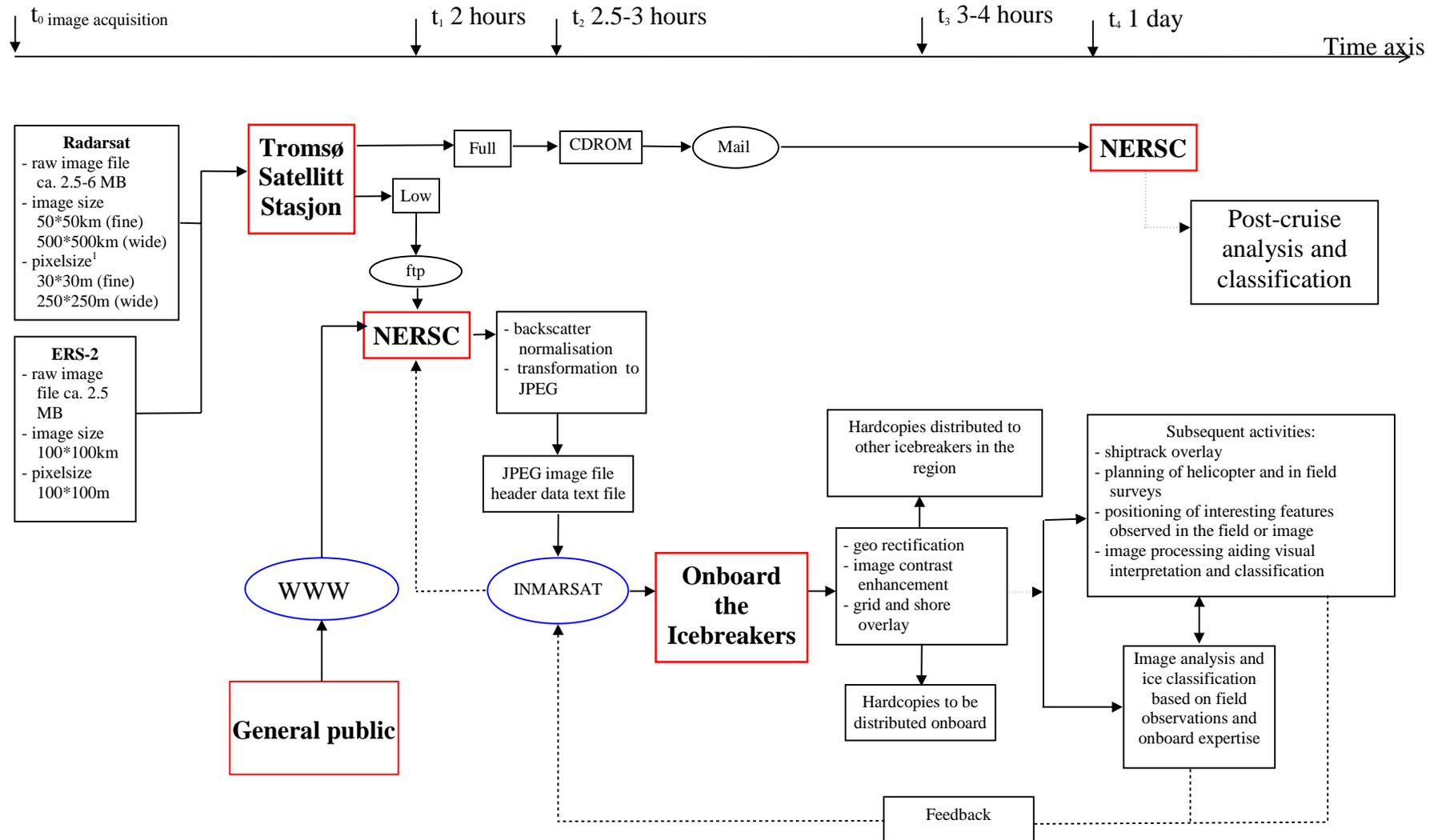
Figure 4. Data float scheme for the SAR images acquired during the ARCDEV expedition.
