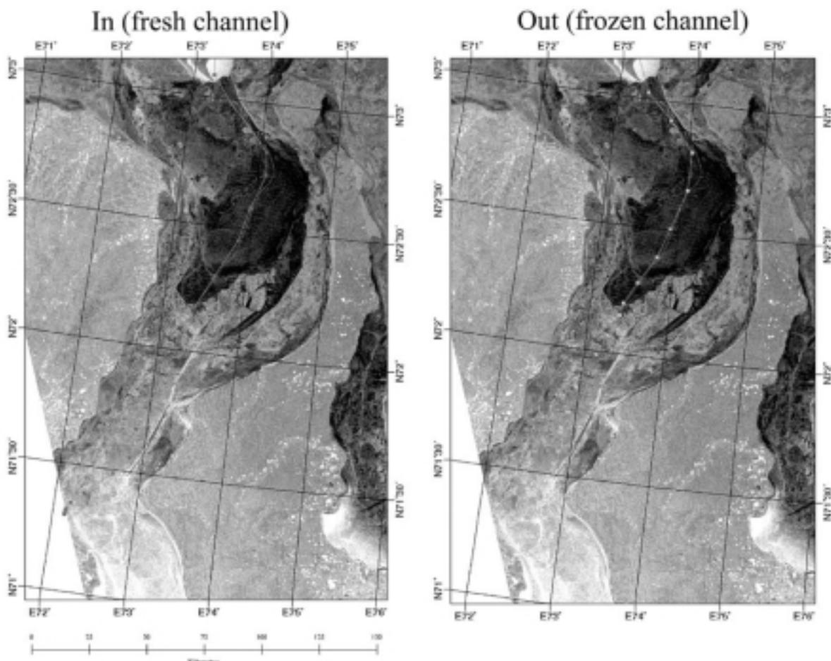
Figure 36. Speed of convoy in and out of Ob estuary. There is one hour between each dot in the two images. The prepared ice channel was frozen, and at certain parts closed, before the return voyage. As it appears, i/b Kapitan Dranitsyn had to struggle to get through the most ridged part of the fast ice (up to 72 °10N).
