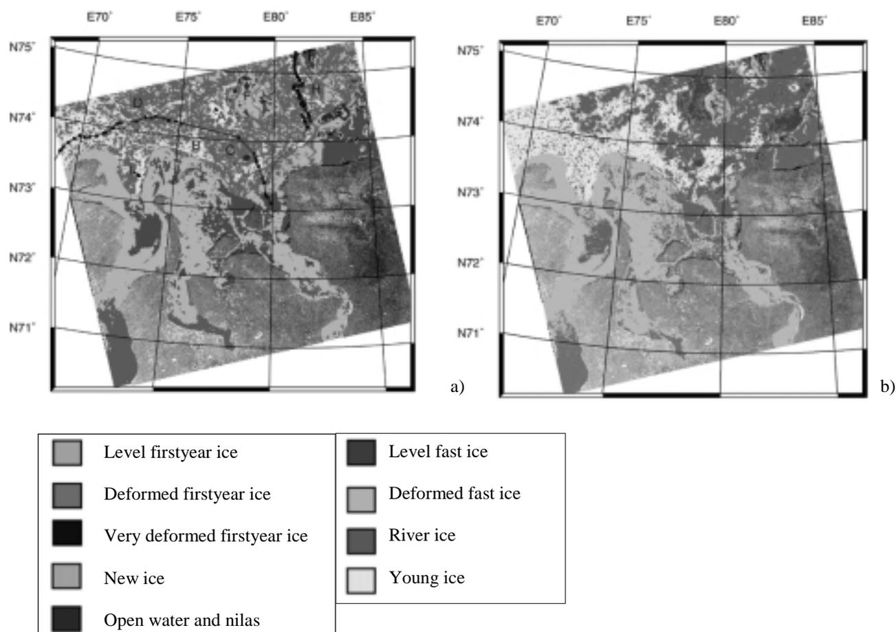
Figure 37. Classification results for the RADARSAT ScanSAR image of April 30, using a) Linear Discriminate Analysis (LDA) and b) Back-propagation Neural Network (BNN).
