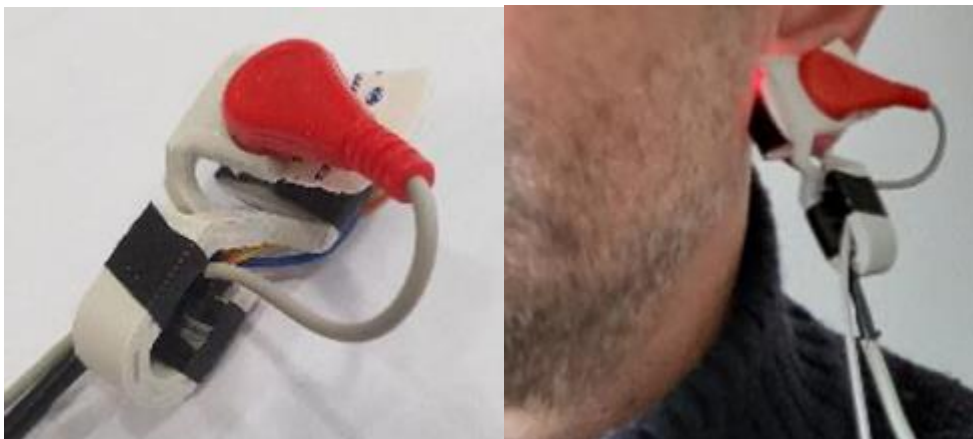
Figure 86. Ear clip with a PPG sensor.
