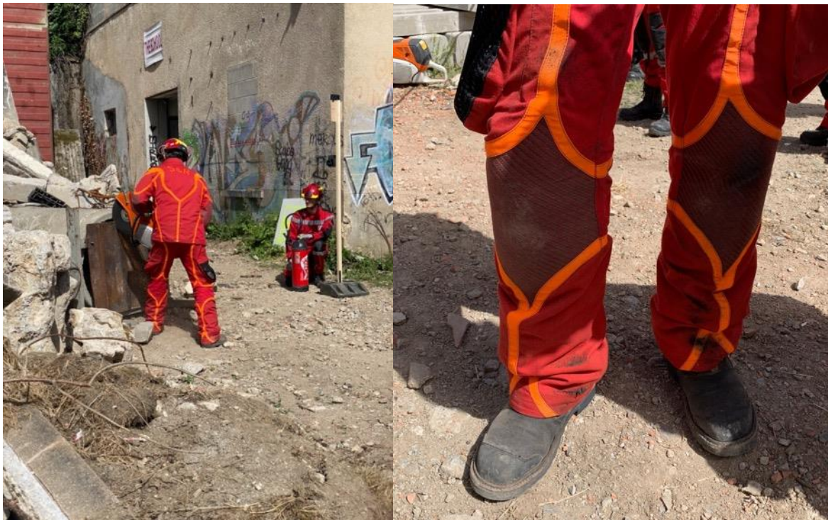
Figure 33. FR wearing the Smart protective uniform during the metal sheet cutting task and the damages in the pants.
