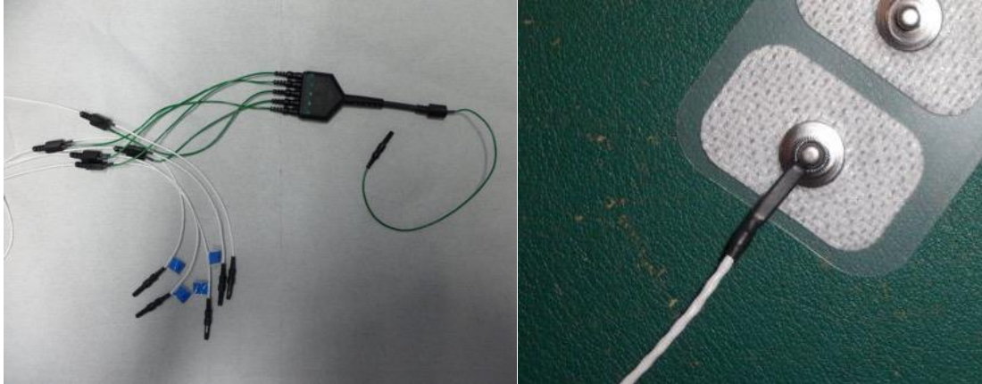
Figure 63. Shielded cables for the ECG recording.
