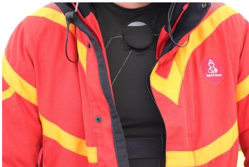
Figure 42. Open male jacket with a detail of the smart underwear (male version).
