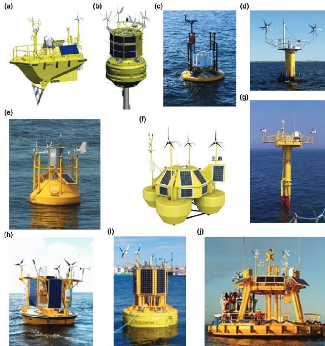
FIGURE 3 | Overview of known floating lidar system realizations—in rows from left to right and top down: (a, b) FLiDAR WindSentinel 6M, 4M, (c) SEAWATCH WindLiDAR Buoy, (d) SeaZephIR, (e) Fraunhofer IWES Wind Lidar Buoy, (f) EOLOS FLS200, (g) FORECAST, (h) DeepCLiDAR, (i) EOLFI BLiDAR, and (j) M 3 EA project. (© figures by system providers as referred to in Table 1)
