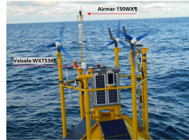
Figure (1) Placement of the atmospheric sensors on the FLS - © Fraunhofer IWES.
