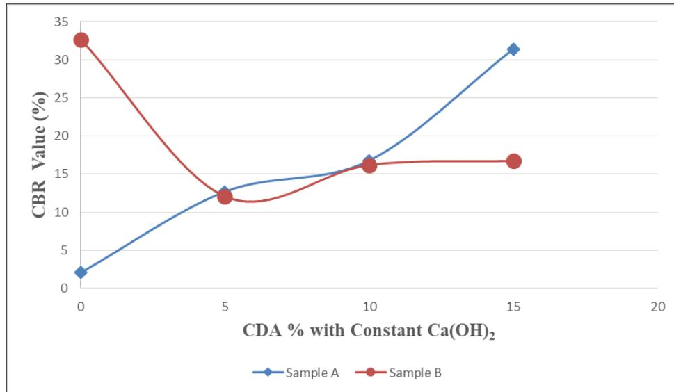
**Figure 3** Variation of Unsoaked CBR with additive content for the two soil samples
