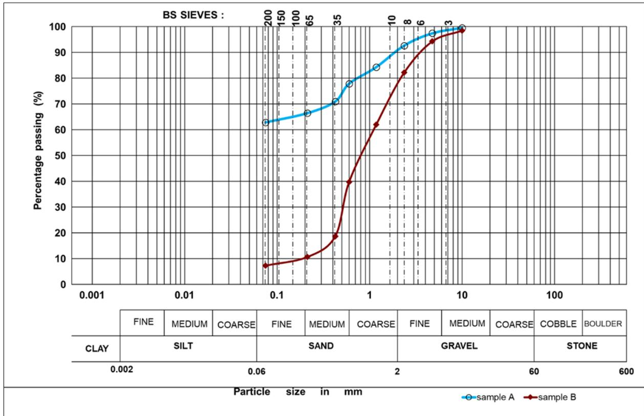
Figure 1 Particle size curve for sample A and B
