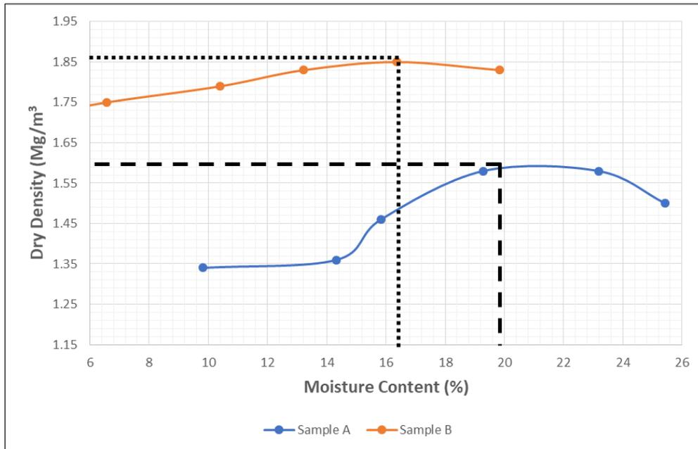
**Figure 2** MDD and OMC graph of the two soil samples
