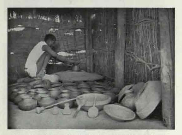
B. Lausadiya: potter at work. Note that the wheel is not spoked but solid. The potter works indoor, Terracotta dabbers, wooden beaters and earthen basins, with which the pots are given the desired shape, are seen in the foreground. See pp. 250 and 251
