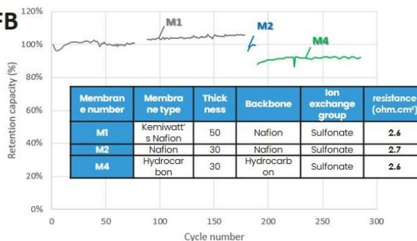
Results: Nafion membrane is chosen due to better stability, Ni foam cannot be used due to increase in manufacturing costs impacting end energy price, new formulation electrolyte is chosen for better AORFB performance.
