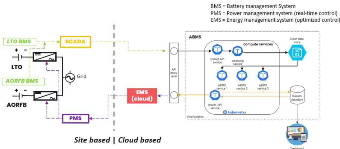
Task 3.3: Optimal electrical architecture of each BESS and the HESS
