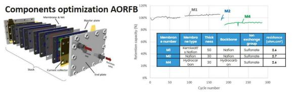
Results: Nafion membrane is chosen due to better stability, Ni foam cannot be used due to increase in manufacturing costs impacting end energy price, new formulation electrolyte is chosen for better AORFB performance.
