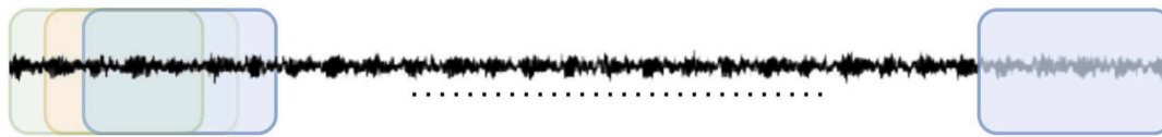
Fig. 5. Data augmentation over raw vibration signal with frame length 400 and step size 20.
