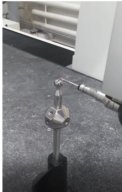
Fig 1. A snapshot of the process of measuring the standard to be checked before starting the measurement.
