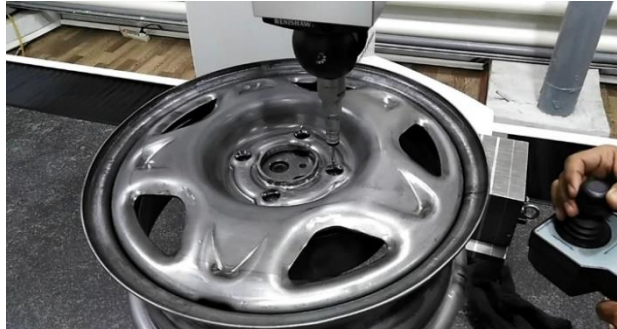
Fig 4. The measurement process of the light car disc part on the coordinate measuring machine.
