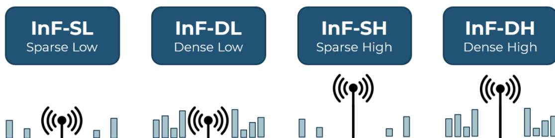
Figure 2.1-1. Indoor Factory (InF) configurations.
