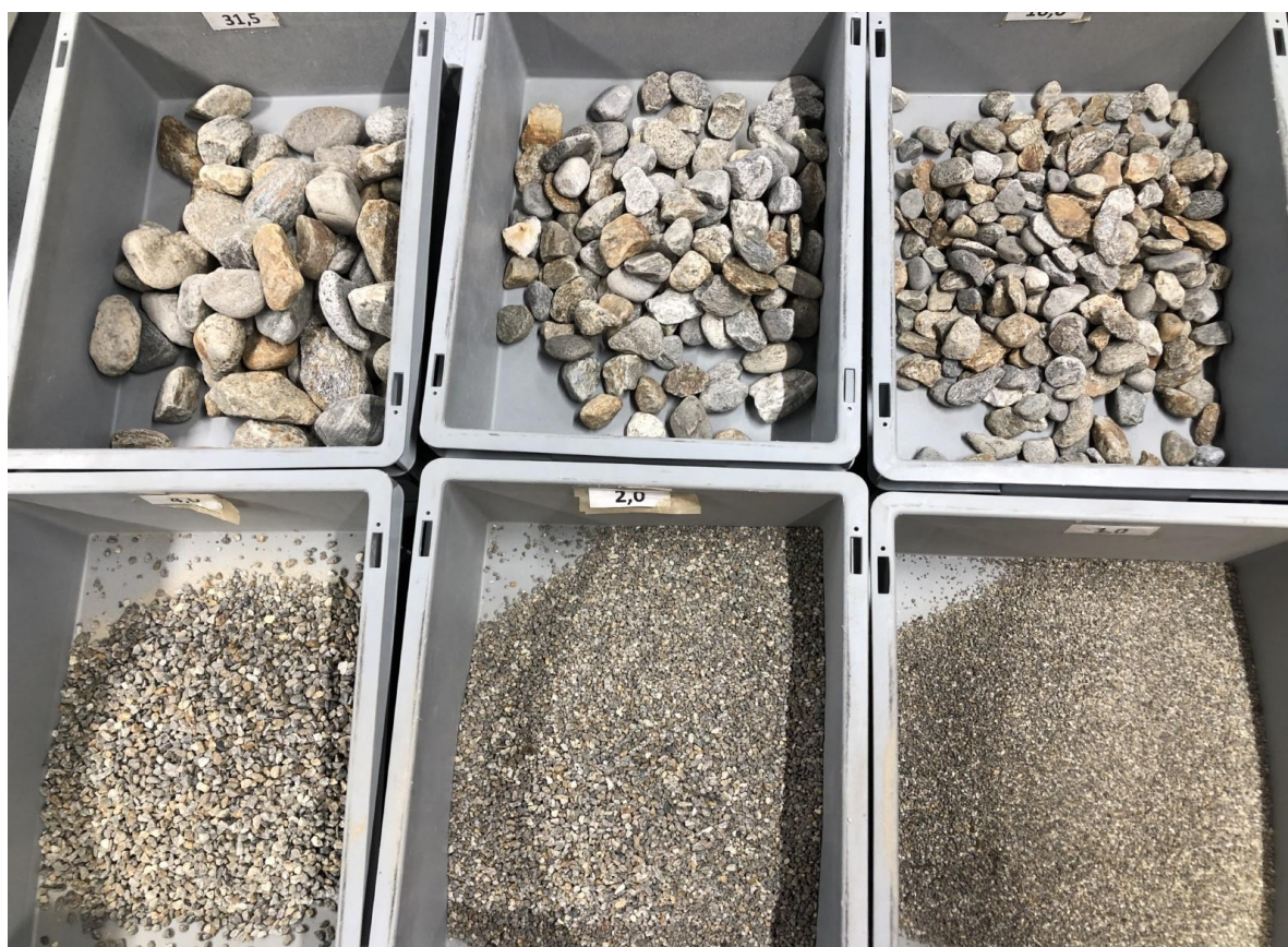
Figure 13. Examples of retained sediment fractions after mechanical sieving.
