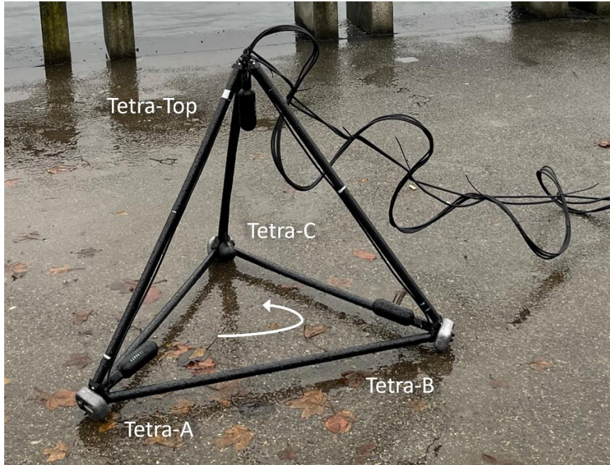
Figure 2. The tetrahedron structure with the four hydrophones mounted inside the corners. The naming convention for the four channels are indicated. The lower three corners are each charged with 1 kg of lead weight. The tetrahedron is suspended with a 5 m long elastic rope to dampen the movements from the surface.
