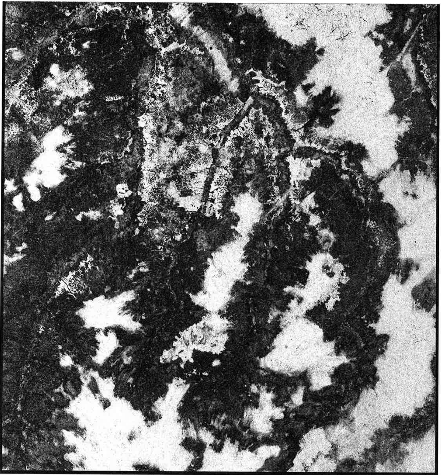
Figure A2. Coherence image generated from two ERS-1&2 SAR images on 30 September 1997 and 1 October 1997.
